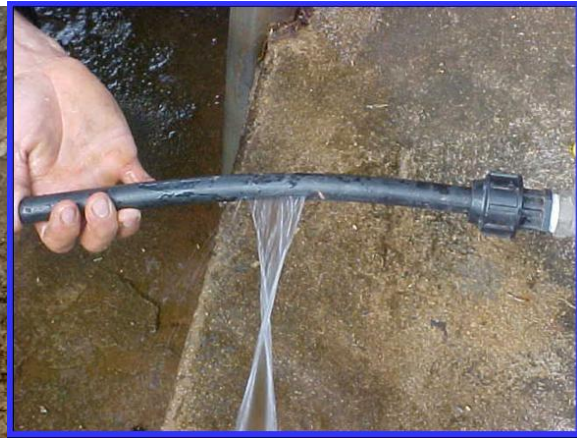
Variable area leaks: splits in flexible pipe materials, background leaks at joints. N1 = 1,5, More sensitive to pressure changes
