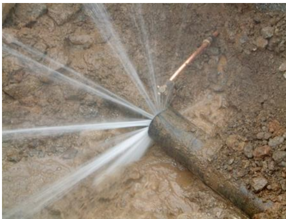
Fixed Area leaks – ring cracks, corrosion holes, blow-outs in rigid pipe materials. N1 = 0,5, Less sensitive to pressure changes
